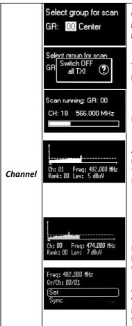
Once started a channel scan operation the receiver asks for group to be used\*. Press and hold the SEL button to select the group to scan.
