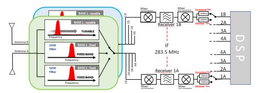
For each antenna the RF signal is split in 4 to receiver 1,2,3 and 4 (antenna A and antenna B) with a wide band splitter. Then 3 banks of filters are selected according to the frequency of the 4 receivers:
